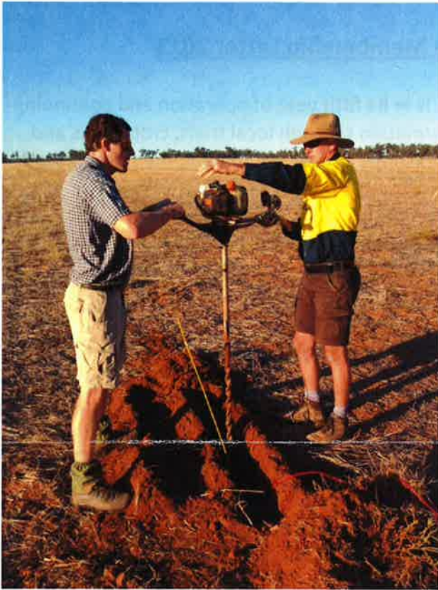
Installation of soil moisture probes, March 2013, a part of Murrumbidgee CMA funding.
